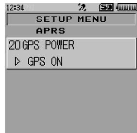
In order to use the GPS satellite data for your own position information, set **[APRS]** → **[24 MY POSITION]** to "GPS". If **[24 MY POSITION]**, is set to "Manual", the coordinates registered in set menu "P1-P10" will be used by your transceiver for APRS operations, and the acquired GPS data will become invalid.
