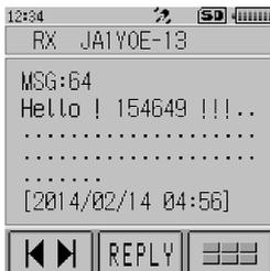
Touch **[F MW]** in the frequency display screen followed by **[M.LIST]** to display the APRS MESSAGE LIST screen.
