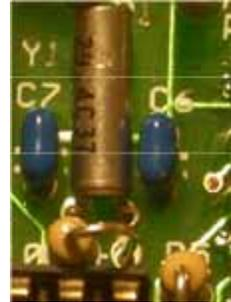
4. Close-up of C6, Y1, C7 – note how inserting Y1 might be tricky if C6 and C7 are both already in place
