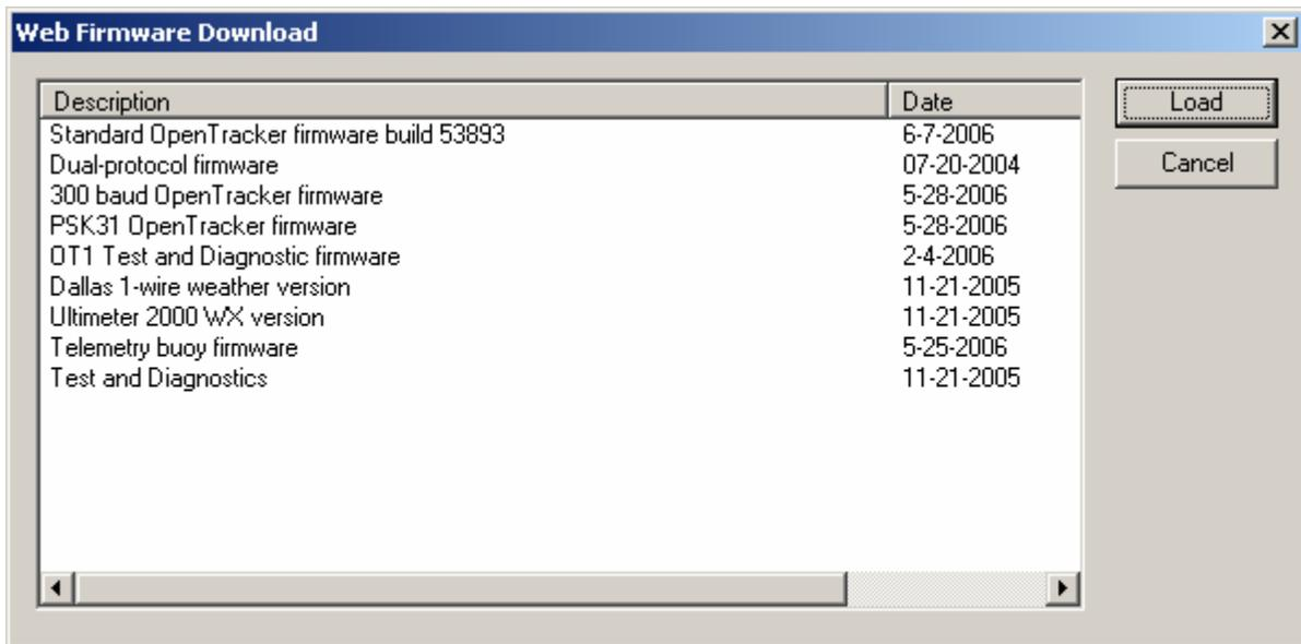
Firmware files are in Motorola S19 format. If you compile your own firmware, the S19 file generated by the linker can be used without modification. Interrupt vectors are automatically rewritten by the configuration program.
