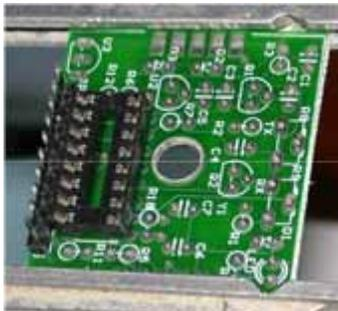
2. Start with microprocessor socket and 10-pin header
