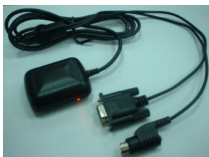
Picture of GPS unit BR304 with connector for RS232 (DSUB) and power (MiniDIN)
