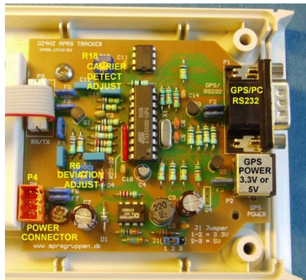
Picture of the completed APRS tracker in enclosure with adjustments points marked
