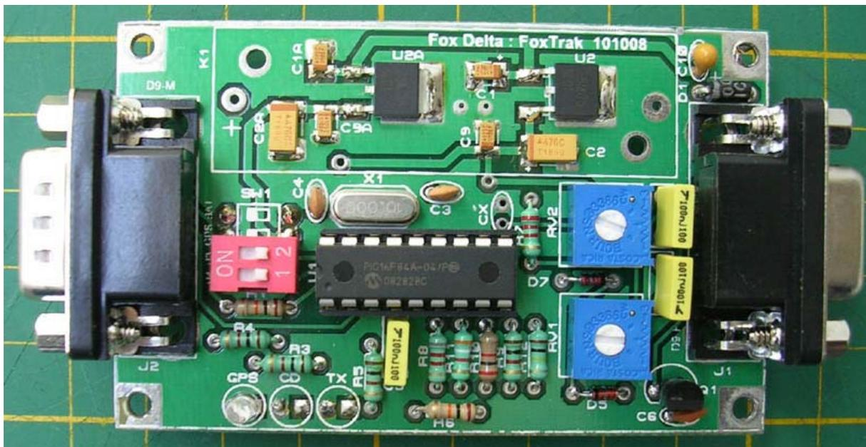
The position data in NMEA format ( \$GPRMC ) delivered from a GPS is decoded and a 1200 bps packet radio signal is generated from it. This can be fed directly into a Radio Transmitter without the need of an expensive TNC. Because of not having enough program memory left on PIC & to make hardware simple, circuit does not decode received APRS signals.
