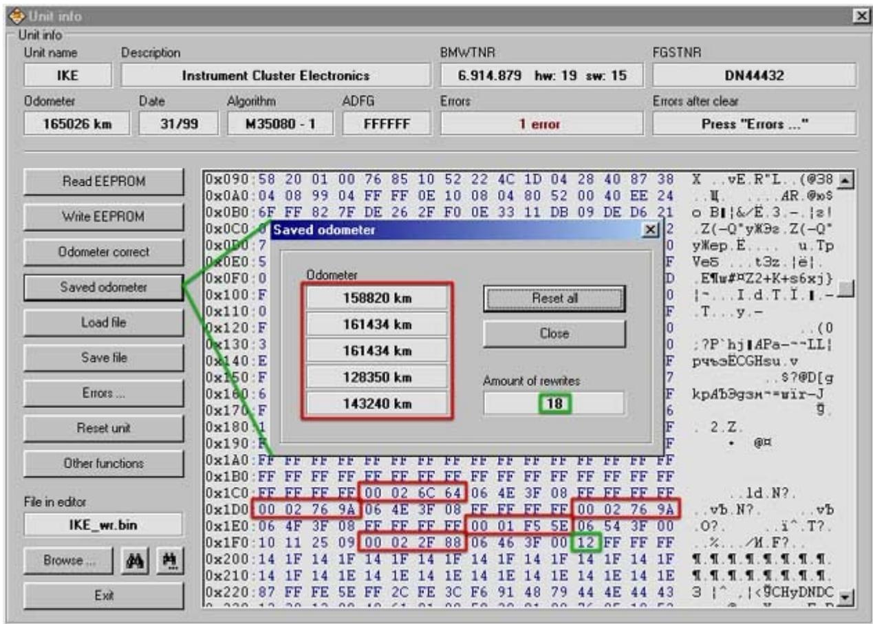
It looks like service data saving method in MB dashboards: serial cycle contains five write procedures + writing counter on #01FC area.
