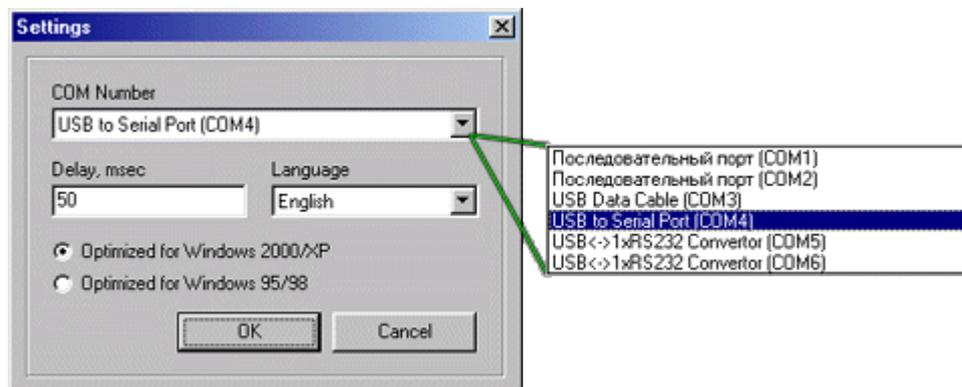
For standart COM port selection in [ COM Number ] field now you can see list of all available COM ports. This list was read from windows registry, so that's no more necessary to select working COM port by checking all of them. All you need to do is only select necessary for you COM port and use it. Its also making virtual COM port detection more easy. Virtual
