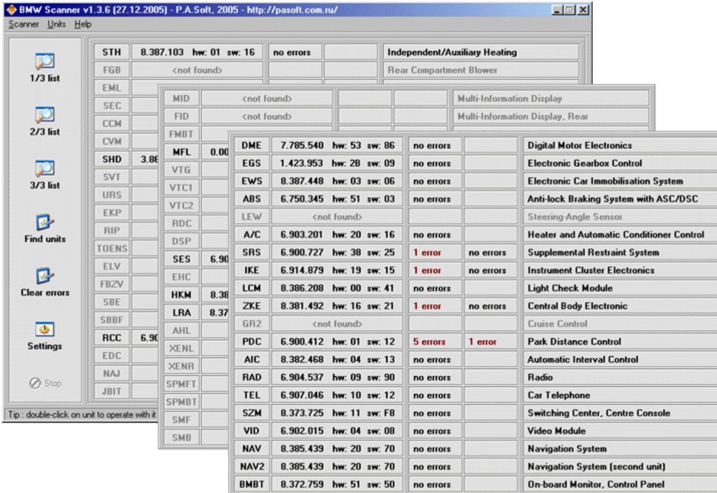
In main menu you can see new [ CLEAR ERRORS ] function. It was cutted from [ FIND UNITS ] procedure. The reason of doing this was a lot of customers asks because in previous versions [ FIND UNITS ] procedure contained also automatically malfunctions codes reset that was making malfunctions analysis more difficult.
