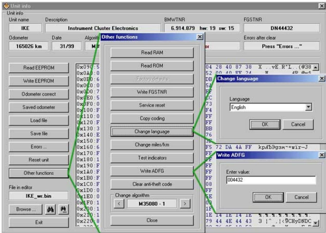
There is different dashboard classification also, using memory access method. For old variant with numbers only (1,2...13) now you can see new classification like: EEPROM memory type + comment (for example 93S56-3, 93S66-Tacho, M35080-E46, etc).
