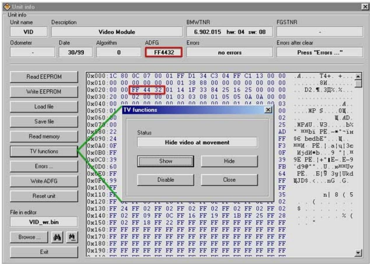
A lot of new functions are available now when work with video module (VID). Added functions like read/write EEPROM memory of unit, software memory reading, and also video when driving settings. This function will help you to set one of 3 possible video settings: show when driving / hide when driving / disable constantly.
